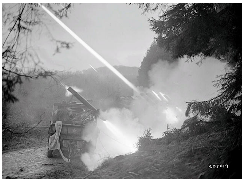
ROCKET ARTILLERY American forces often used local artillery to stop German counter-attacks. These are GMC trucks near Bergstein with two T27 eight-barrel rocket launchers. Despite its fearsome launch, the M8 rocket was inaccurate and the Americans eventually copied a German version. NATIONAL ARCHIVES
